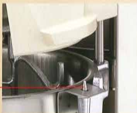
2 : Fit bowl supports over locating pins
